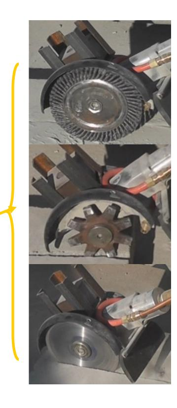
Wire Brush Cleaning Cracks
