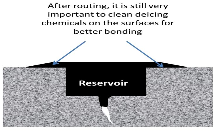
**Elevation view of routed crack after sealing**
