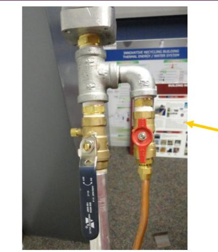
**Adjustable Air Flow Splitting Design** One for running motor, the other for air blasting to clean debris
