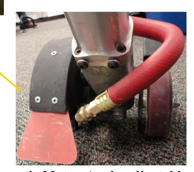
Pneumatic Motor, Angle-adjustable air nozzle. and Debris Guard The debris guard is not only for the safety and protection o the operator, but also for passing vehicles and pedestrians. The adjustable nozzle trajectory using a funnel to blow out debris away from the crack to the side of the roadway no
