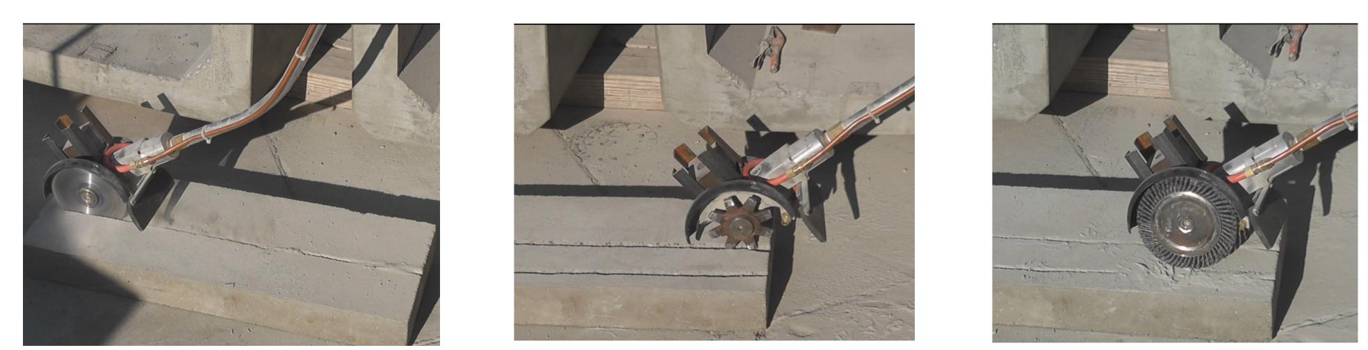
Versatile functions provided by a single pneumatic powered device developed in this project
