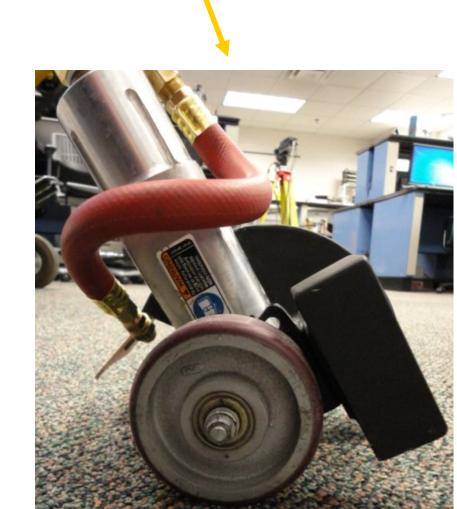
**Guiding Wheel with Height** Adjustable Assembly Give the operator a choice in the setting the minimum crack depth
